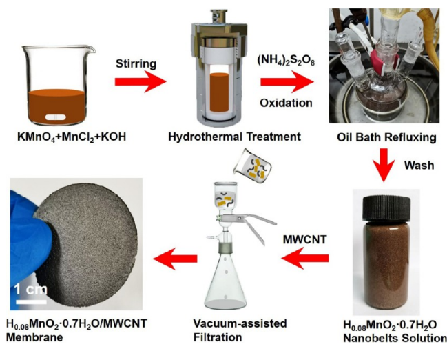
Scheme 1. Schematic Illustration of the Fabrication Process of Macroporous, Freestanding \text{H}_{0.08}\text{MnO}_2 \cdot 0.7\text{H}_2\text{O} /MWCNT Membrane
