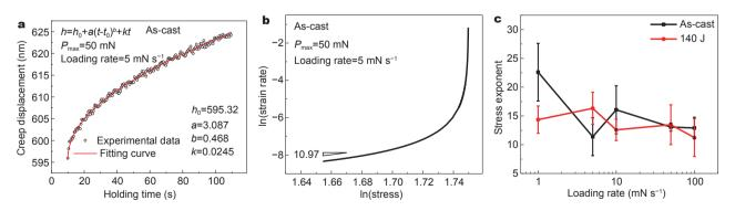
Figure 4 (a) The typical experimental and fitted creep curves of the as-cast  $Zr_{35}Ti_{30}Cu_{8.25}Be_{26.75}$  MG at a loading rate of 5 mN s<sup>-1</sup> by using the Kelvin model. (b) The ln(strain rate)-ln(stress) plot. (c) Steady-state stress exponent, *n*, of the as-cast and ultrasonic-oscillated MGs as a function of indentation loading rates. The solid lines are guides for the eyes.
