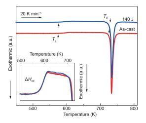
**Figure 1** DSC curves of the ultrasonic-vibrated  $Zr_{35}Ti_{30}Cu_{8.25}Be_{26.75}$  MG with the applied energy of 140 J at a heating rate of 20 K min<sup>-1</sup>. The data for the as-cast sample were plotted for comparison. The inset shows the enthalpy recovery measurement.
