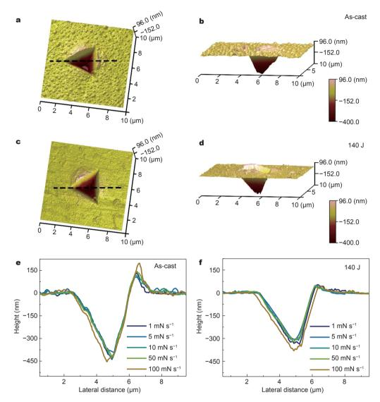
Figure 3 AFM images of the as-cast (a, b) and 140 J ultrasonic-vibrated (c, d)  $Zr_{35}Ti_{30}Cu_{8.25}Be_{26.75}$  MGs after nanoindentation at a loading rate of 5 mN s<sup>-1</sup>. The cross profile of the indents after nanoindentation for the as-cast (e) and 140 J ultrasonic-vibrated (f) samples.
