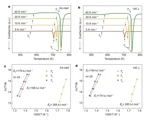
**Figure 6** Thermodynamic and kinetic characteristic parameters of the  $Zr_{35}Ti_{30}Cu_{8.25}Be_{26.75}$  MG samples. DSC traces of the as-cast (a) and 140 J ultrasonic-vibrated (b) MGs at heating rates ranging from 5 to 40 K min<sup>-1</sup>. Kissinger plots of the as-cast (c) and 140 J ultrasonic-vibrated (d) MG samples to calculate the activation energies relative to  $T_{e}$ ,  $T_{x}$ , and  $T_{p}$ , respectively, and the fragility parameter *m*.
