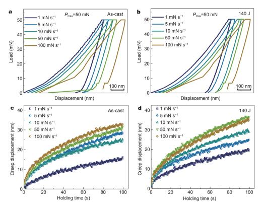
**Figure 2** Creep behaviors of the  $Zr_{35}Ti_{30}Cu_{8.25}Be_{26.75}$  MG samples. (a, b) Load-displacement (*P*-*h*) curves under different loading rates of the as-cast (a), and 140 J ultrasonic-vibrated (b) samples. The curves in (a) and (b) offset from the origin for clear viewing. (c, d) The creep displacement of the as-cast (c) and 140 J ultrasonic-vibrated (d) samples during load holding period under different rates.
